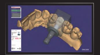
With the help of exocad ChairsideCAD, crowns, inlays, onlays, veneers and small bridges can be designed and manufactured directly at the treatment center in a very innovative and fast workflow. Using the integrated In-CAD Nesting module, the designed jobs can be placed directly in the block for calculating and milling by the machine.
