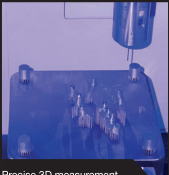
Precise 3D measurement in the CORTEC 650i
