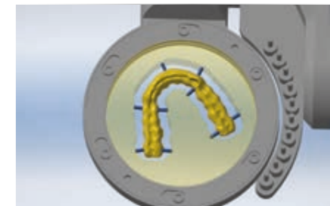
Bite splint made of PMMA in blank holder
