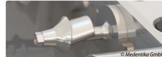
Preshaped abutment fixed inside the machine
